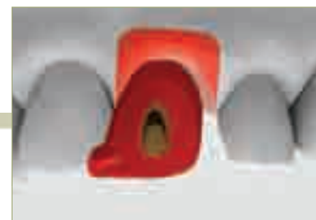
Modify Angled abutment properly and fabricate positioning jig
