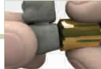
Eliminate the Lip remnant caused by 'snap-on' mechanism by reamer
