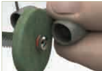
Trim extended margin by rubber wheel
